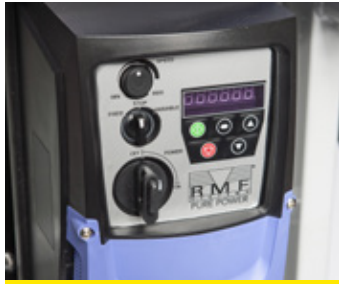
FREQUENCY CONTROLLER Regulates the speed of the electric motor and display actual amperage, RPM and frequency.
